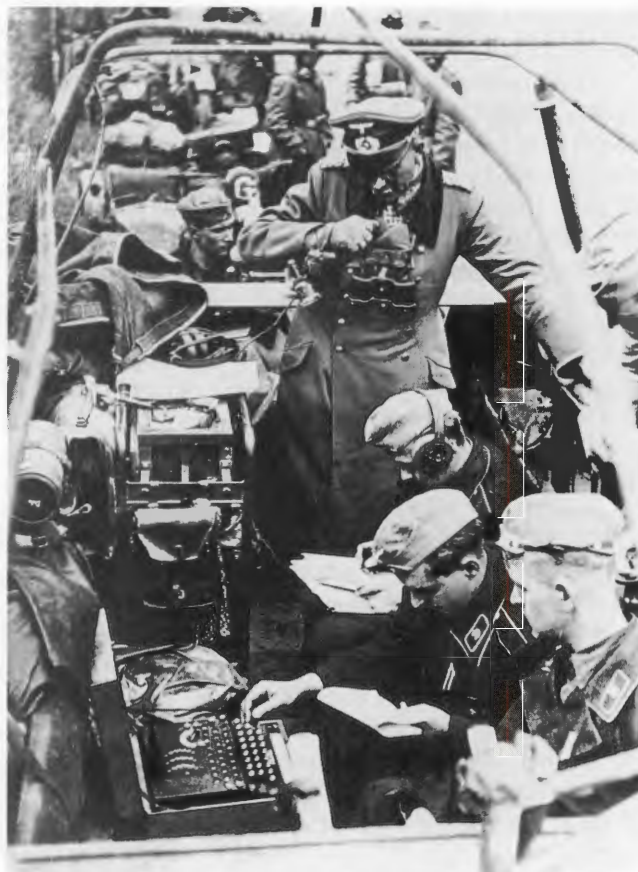
The Enigma Machine During World War II, German armed forces used Enigma machines like the one seen here in the vehicle of a German tank commander. With Enigmas, they could encrypt and decode radio messages, keeping them secret (they believed) from enemy code-breakers. (Brian Johnson)
