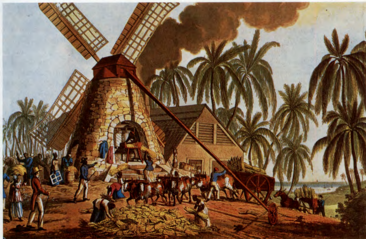
Caribbean Sugar Mill The wind mill crushes sugar cane whose juice is boiled down in the smoking building next door.
